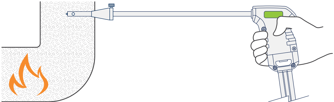
Fig. 3-6: Probe Placed in Center of Measurement Area
