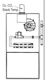
Combustion testing of fan assist or power vented, furnaces/boilers should be done through a hole drilled in the vent immediately above the inducer fan.
