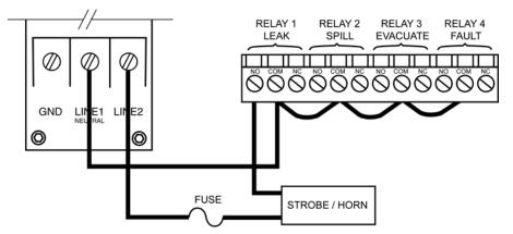
Jumper the 'Neutral' line of an external power source or the monitor's AC input to the 'Common' terminals on the relay connector.
