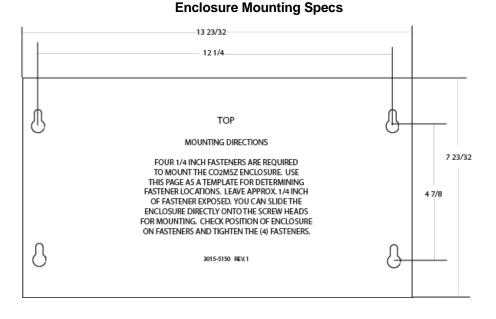
Hold the monitor flat against the mounting surface and allow it to slide down engaging the screw heads in the keyhole slots of the mounting brackets. Adjust the screws as necessary to hold the monitor securely against the mounting surface.
