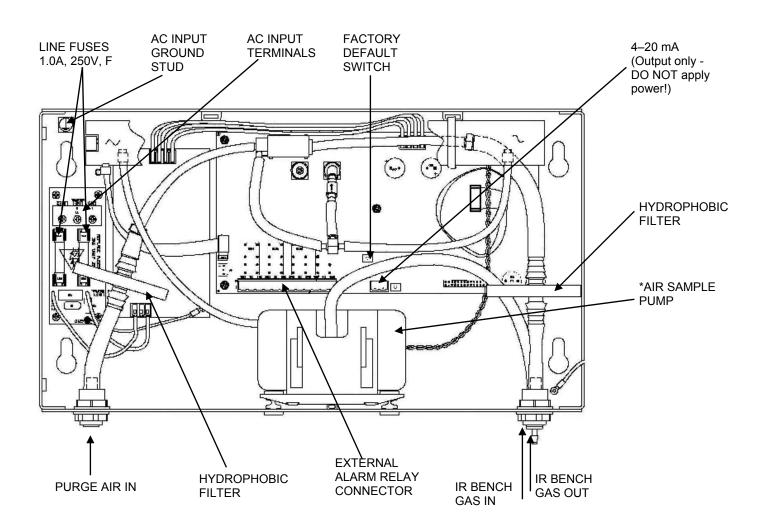
\***NOTE**: The plastic cable tie surrounding the air pump is to ensure safe handling during shipping. Please remove before operating.
